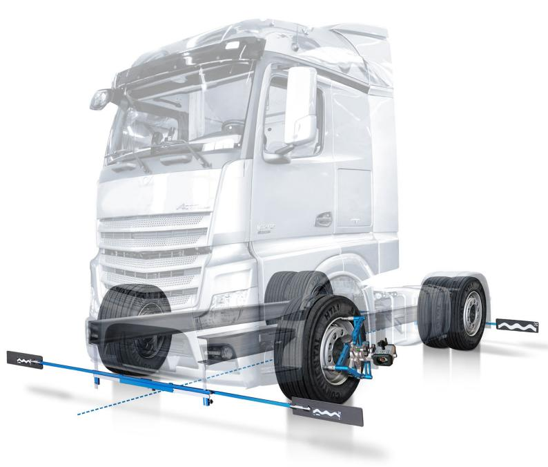
**THE SYSTEM** is designed to measure commercial vehicles like trucks, trailers, buses and light commercial vehicles. Each axle is measured individually by using the rolling method or measured after Run-out compensation.
