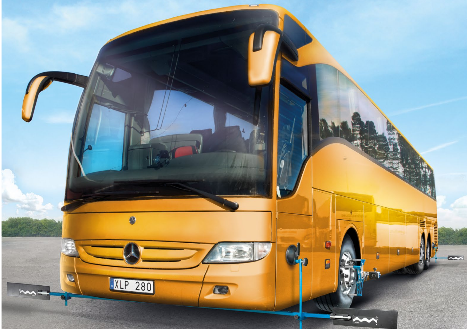
Bus attached with TC-126 Bus and Van kit, TC-175 Wheel Adapter Spider and TC-256 Camera Sensor.
